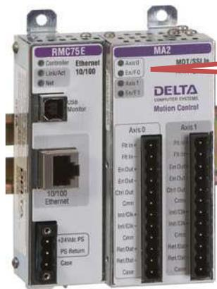
After the download ensure that there are NO FAULTS on the Module. RED LED indicates a FAULT.
